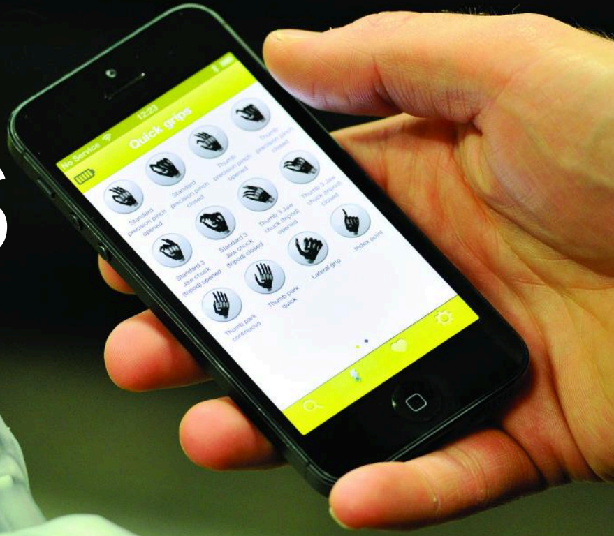
The i-Limb Ultra Revolution can be operated via an iPhone app that gives the wearer greatly expanded control capability
